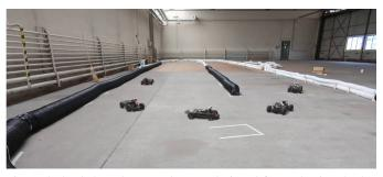
Figure 4. Oval-shaped racetrack setup designed for evaluating the lap times of various sensor configurations. The track is characterized by its distinct half-and-half boundary, composed of a black, ill-reflectivity sector and a white, well-reflecting one.
